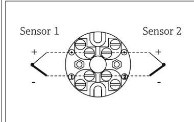
Wire specifications: Thermocouple grade, TFE insulated 20AWG, 7 strands with stripped ends
