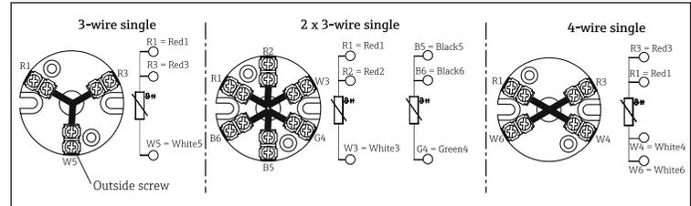
**i** The blocks and transmitters are shown as they will sit inside the heads in reference to the conduit opening. ALWAYS terminate leads to the outside screw!
