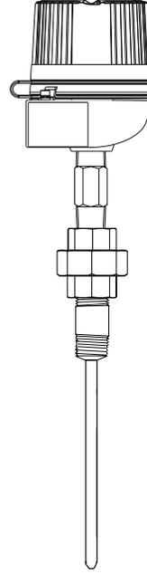
The Pt100 RTD is specifically designed for use in two different process temperature ranges:
