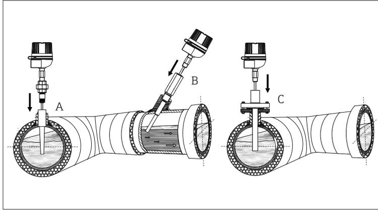
Examples of spring loaded insert installation.
