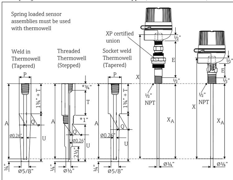
\*For thermowells with 1/2" NPT - 1" Process thread length and 3/4" Hex length dimensions are reversed.
