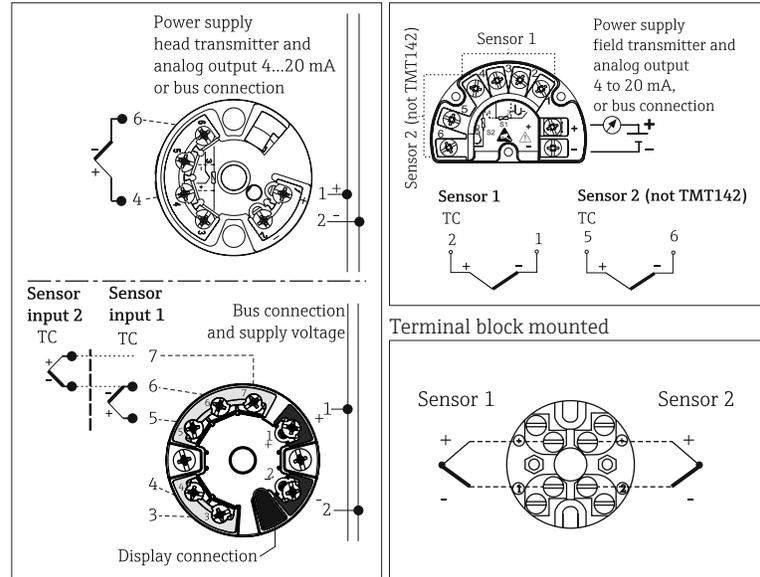
Wire specifications: Thermocouple grade, TFE insulated 20AWG, 7 strands with stripped ends
