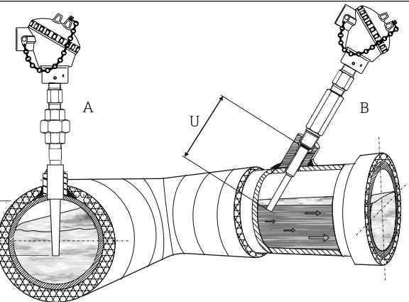
Examples of pipe installation. In pipes of a small section the axis line of the duct must be reached and if possible slightly exceeded by the tip of the probe (=U).
