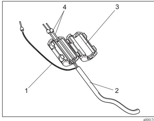
Fig. 15: Interference protection of the signal cable
