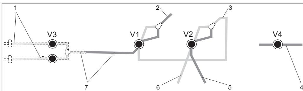
Fig. 9: Valves and valve hoses CA71SI-A
