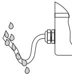
The cables must loop down before they enter the cable entries ("water trap").
