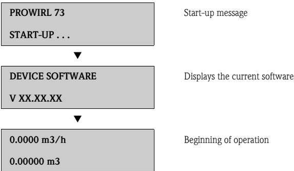
The measuring device starts operating as soon as the startup procedure is complete. Various measured values and/or status variables appear on the display.
