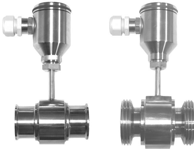
The TR 46 is a temperature sensor specifically designed for hygienic applications (mainly in the pharmaceutical field). It is designed to avoid any intrusion of the measurement probe into the process duct.
