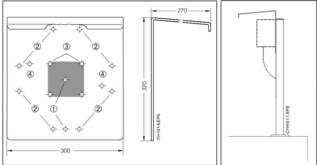
Fig. 3.9 Weather protection cover CYY 101 with Mycom CLM 151 mounted on upright post
