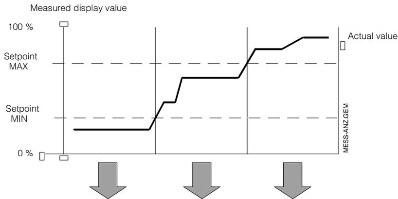
Fig. 6.8: Status diagram for automatic operation of Mycom CLM 151 with limit contacter function
