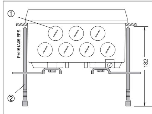
Fig. 3.4: Bottom of field housing with straining screws installed for panel mounting
