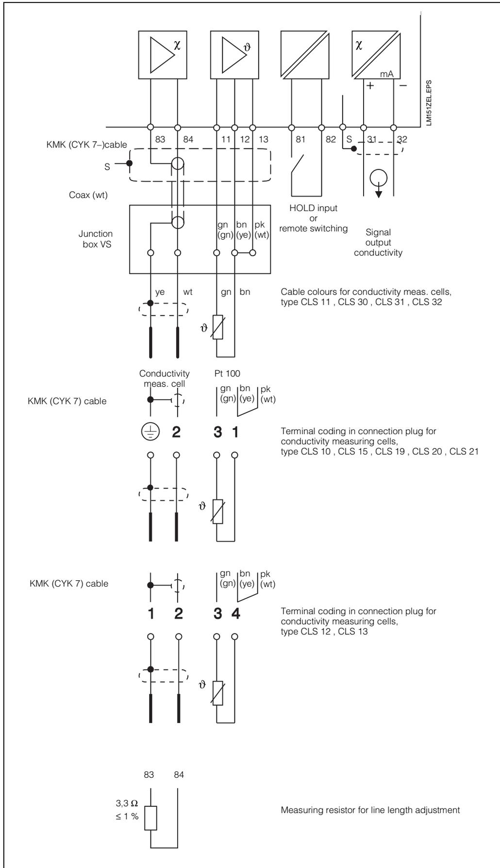
Fig. 4.6: Connection of 2-electrode conductivity measuring cells to Mycom CLM 121 / 151
