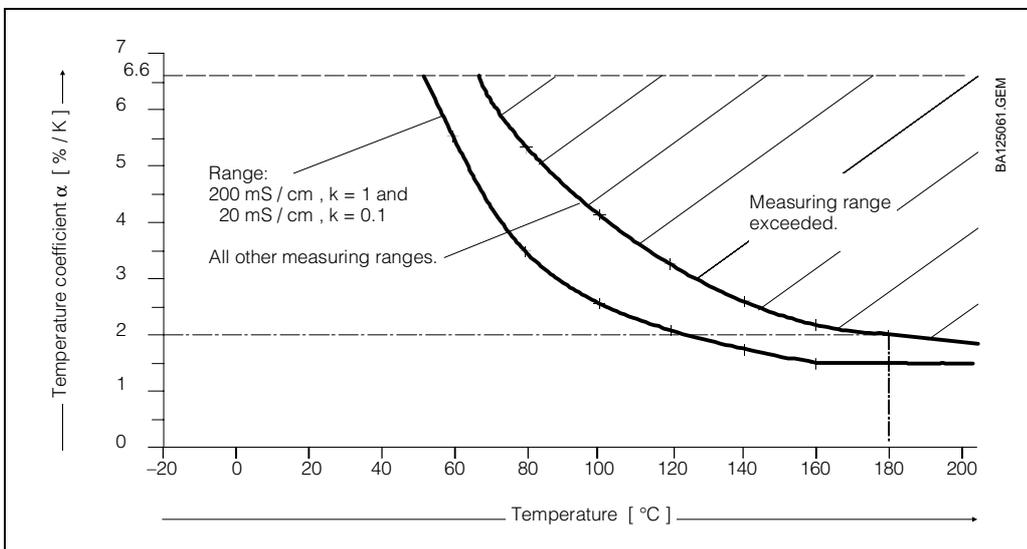
Fig. 6.4: Limit curves for temperature coefficient values; reference temp. 25 °C
