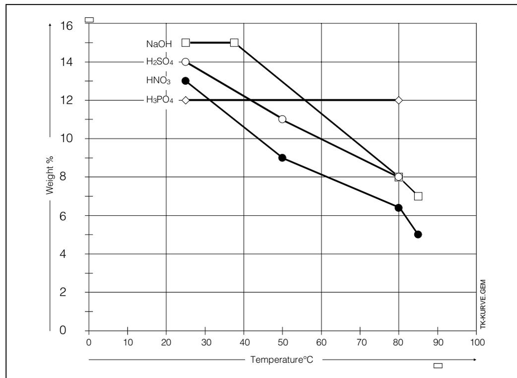
Fig. 6.6: Limit curves for concentration measurement within working temperature range
