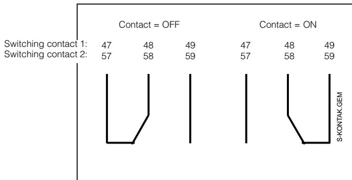
Fig. 6.9: Contact positions for switching contacts with terminal assignments (acc. to fig. 4.2, chapter 4.4)
