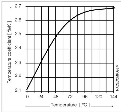
Fig. 6.2: Dependence of the temperature coefficient over the concentration of different electrolyte solutions; reference temperature 25 °C
