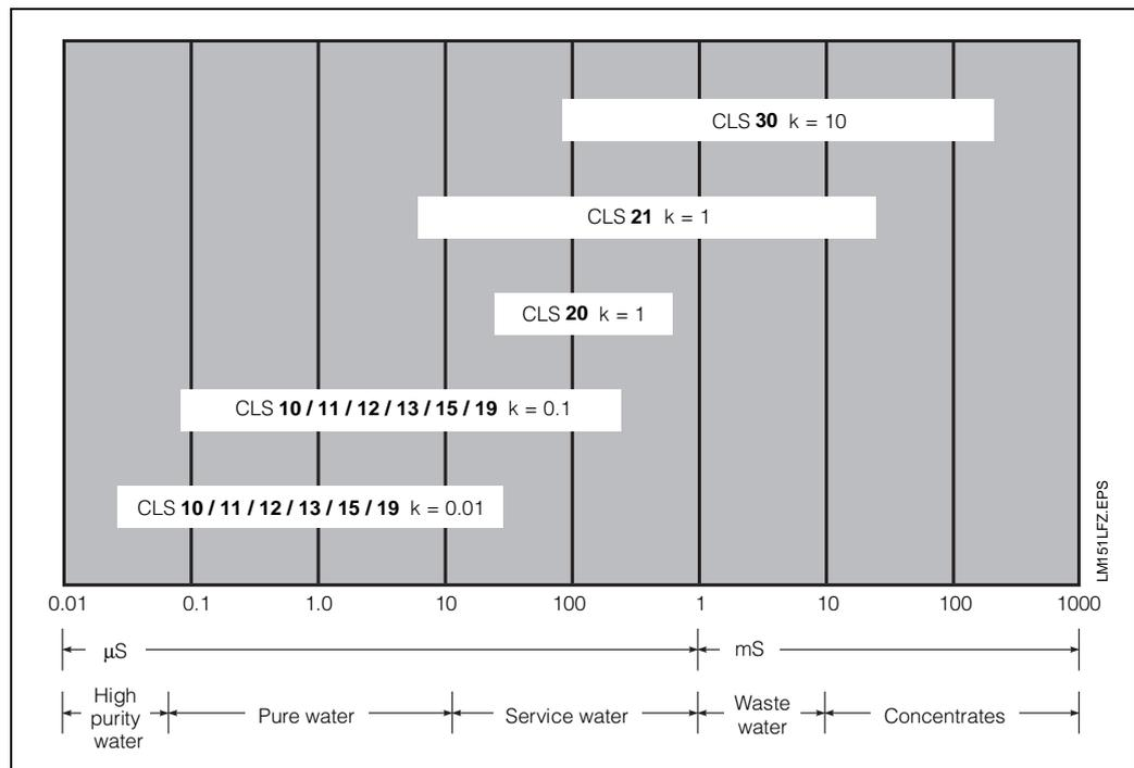
Fig. 5.1: Areas of application for conductivity measuring cells
