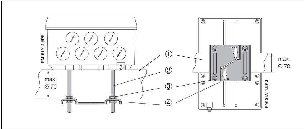
Fig. 3.6: Installation of field housing on horizontal tubing
