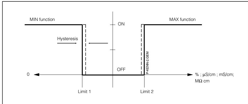
Fig. 6.7: Characteristic curve of limit contactor
