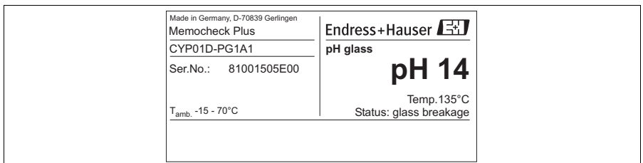
Fig. 9: Memocheck Plus CYP01D nameplate example (pH glass electrode, value: pH 14)
