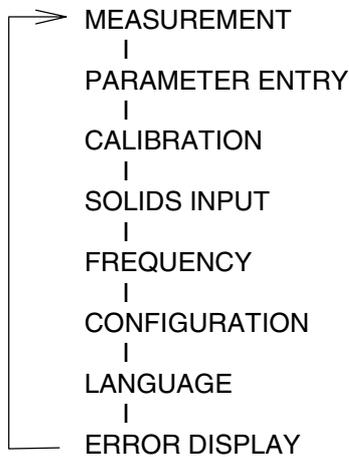
After the instrument is powered on, it switches automatically into the measuring state. By pressing the “M” key you get the main routine MEASUREMENT (same from almost any main routine or sub routine). If the measurement program is not automatically started after switch on (e.g. if the system has not been configured yet), press the “M” key before turn on and until the word MEASUREMENT is shown on the LCD display.
