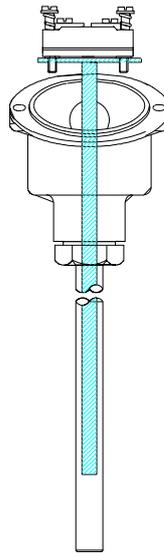
Thermocouples are used for temperature measurements in the range from  $-250\text{ }^{\circ}\text{C}$  to  $+2200\text{ }^{\circ}\text{C}$
