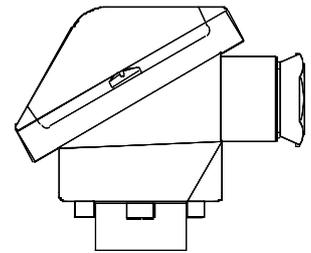
Fig 2 - Terminal head conform to DIN 43729 type B
