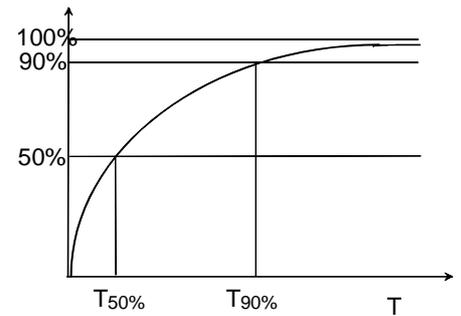
Fig 1 - Graphic representation of the response time inserted in the TSC thermometer Technical Information
