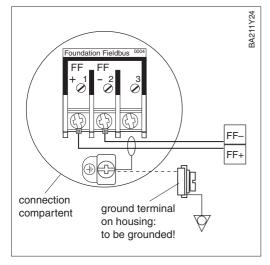
The bus line also carries power and is **Cable connection** connected as follows:
