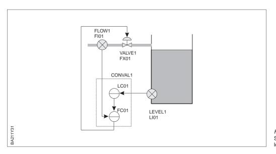
*Figure 3.6* Schematic diagram of control loop
