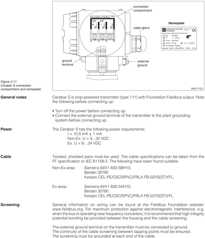
If there are large differences in potential between grounding points, the grounding should run via a capicitor that is suitable for high frequency use
