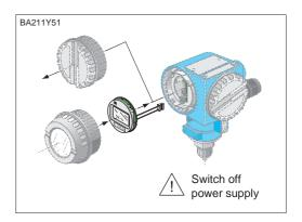
• Insert the plug of the display in the centre jack. Note the coding of the plug and jack.
