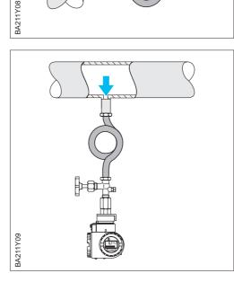
Figure 2.2 Mounted with U-shaped pigtail for measuring steam/vapour
