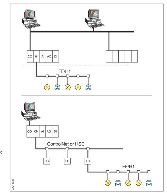
*Figure 3.1* Foundation Fieldbus principle of operation
