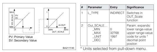
If the display and the OUT value of the analog input block are to provide the same value, then the lower and upper limits of the XD\_SCALE value during calibration or linearization must be entered as the lower and upper limits of the OUT\_SCALE value (default = 0% and 100%).
