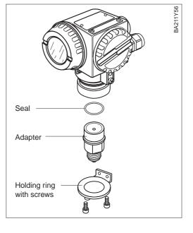
The diagram on the next page shows all replacement parts, together with their order numbers, which can be ordered from Endress+Hauser.
