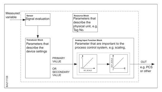
*Figure 3.3* Block model of device
