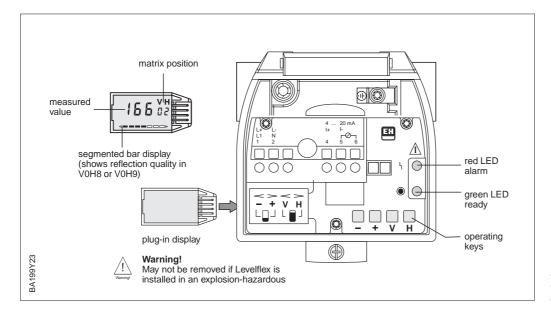
Fig. 4.1 Operating elements of the Levelflex FMP 232 E/332 E
