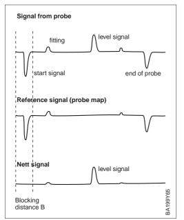
Levelflex senses discontinuities not only within its surroundings but also within the probe itself. This means that each probe has a characteristic signal spectrum, even when it is operating under ideal conditions. This spectrum is recorded before delivery and stored as a reference signal, the so-called factory probe map.
