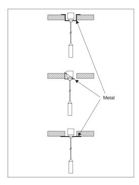
If the Levelflex is to be installed in a thick concrete bunker, for example, then the front face of the process connection should be flush with the inside of the bunker roof. The figure shows installation examples.
