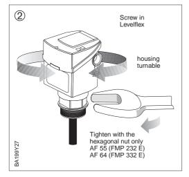
Screw the Levelflex into the process connection or to flange.
