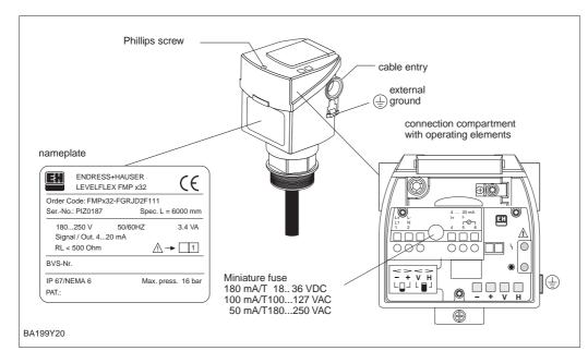
Levelflex is a four-wire transmitter with active 4...20 mA analogue output and optional HART signal. Note the following before connecting up the device:
