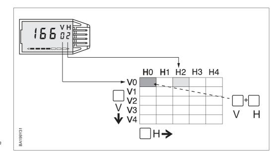
Fig. 4.2 Matrix operation with plugged in display
