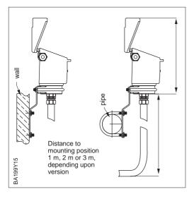
The ambient temperature at the probe head may not exceed +70 °C. For the Dust-Ex version the limit is +60 °C (check the certificate)
