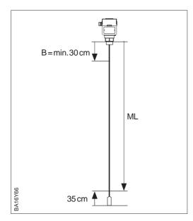
The distance from the top thread to the end of the zone in which signals can be reliably detected is the measuring length ML. This is automatically calculated when a probe map is made by subtracting 35 cm from the position of the end of probe signal. When delivered from the factory, the empty distance E is set equal to ML.
