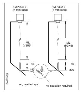
The probe must be anchored as close as possible to the bottom of the silo, e.g. to a suitably dimensioned welded eye.
