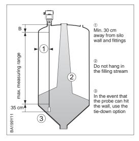
Levelflex is mounted at the top of the silo, ideally in a  $1\frac{1}{2}$ " socket. It requires that the probe rope is hung, *fully extended*, across the entire distance where level measurement readings are desired.
