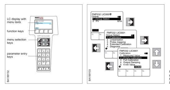
Fig. 4.3 Operating elements and key functions of the HART handheld DXR 275
