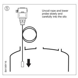
Uncoil rope and lower it slowly and **Inse** carefully into the silo.
