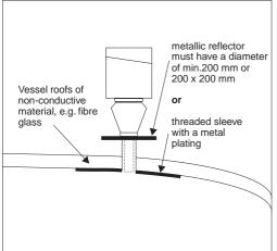
The sensor must be installed in a metal part to act as a reflector when it is installed in a plastic or wood silo. This can be a flange from DN 100mm/4" or larger, or a reflector similar to that shown in the following picture:
