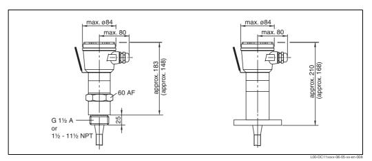
left: Multicap DC 11 with threaded boss and gas-tight gland right: Multicap DC 11 with flange and gas-tight gland
