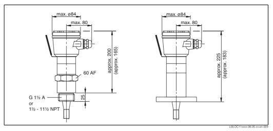
left: Multicap DC 11 with threaded boss and temperature spacer right: Multicap DC 11 with flange and temperature spacer
