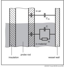
Simplified circuit diagram showing capacitance measurement with fully insulated probes
