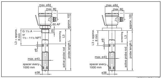
left: Multicap DC 11 with threaded boss, screening and ground tube right: Multicap DC 11 with flange, screening and ground tube
