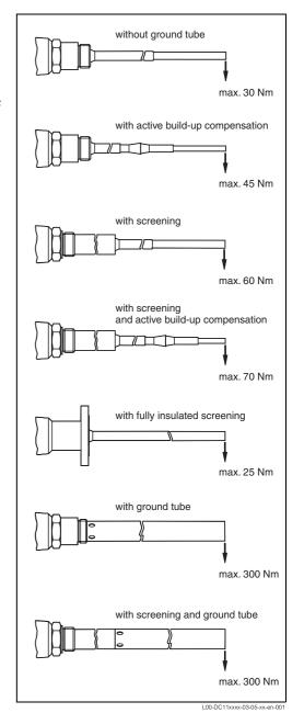
Lateral load bearing capacity for the probe at 20 °C (70 °F) and static load
