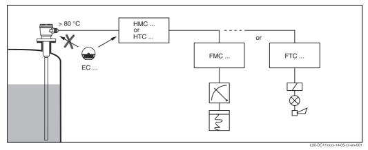
Separate mounting of the electronic insert with an excessively high ambient temperature for the probe head housing
