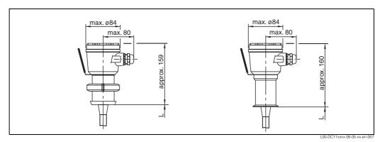
left: Multicap DC 11 with sanitary thread DIN 11851-DN 50 right: Multicap DC 11 with 2" Triclamp coupling
