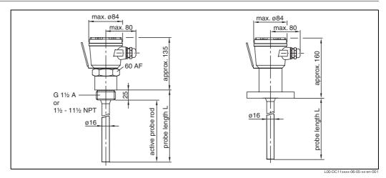
left: Multicap DC 11 with threaded boss right: Multicap DC 11 with flange
