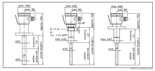
left: Multicap DC 11 with PTFE covered flange and fully insulated screening middle: Multicap DC 11 with threaded boss and screening right: Multicap DC 11 with flange and screening
