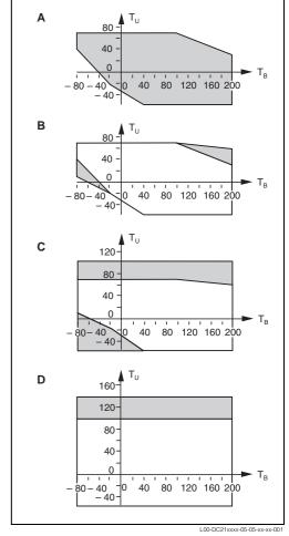
Application range of the various types as a function of operating and ambient temperature
