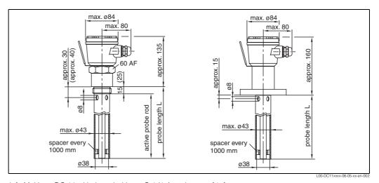
left: Multicap DC 11 with threaded boss G 1 ½ A and **ground tube** (Dimensions in brackets are for the threaded boss with 1 ½ -11 ½ NPT) right: Multicap DC 11 with flange and **ground tube**
