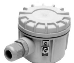
K Synthetic housing in PBTP with »water-tight« cable gland PG 16, Protection IP 66
