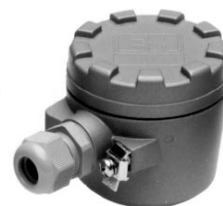
R Aluminium housing with synthetic coating, for aggressive atmospheres; with »water-tight« cable gland PG 16, Protection IP 66
