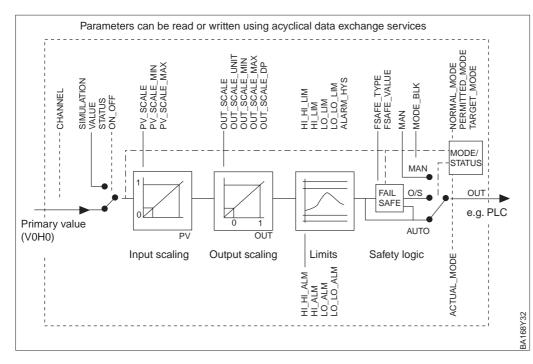
Figure 3.4 Schematic diagram of the Cerabar S analog input block
