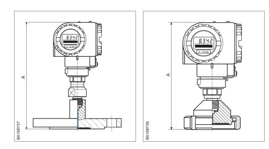
Figure 9.2 left: Cerabar S PMP 635 with flange or thread
