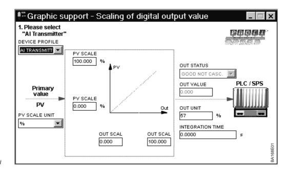
Figure 3.7 Scaling of the Out Value via graphic support in Commuwin II
