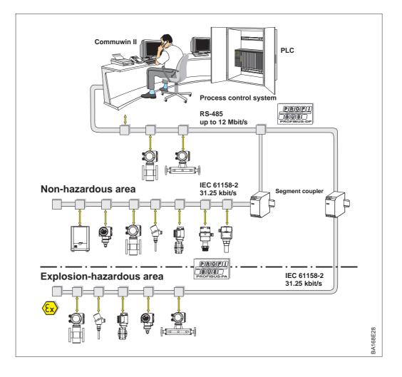
Figure 3.1 PROFIBUS-DP/-PA principle of operation
