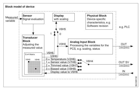
Figure 3.3 Block model of the Cerabar S with PROFIBUS-PA profile 3.0
