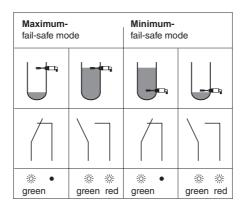
The symmetrical vibrating fork is excited to its resonance frequency which changes when the fork is submerged in liquid. The change is registered by the electronics, which actuate an electronic switch at the PNP output.
