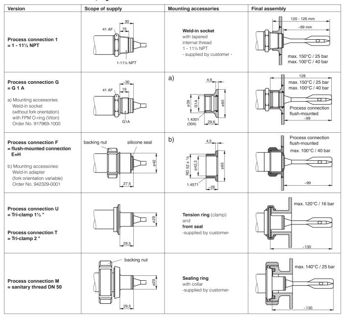
The specified limits for temperature and pressure apply in each case to the limit switch with special process connection Also note the limits for the seal and clamping ring used!
