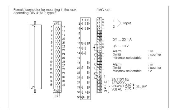
Fig. 5.3 Pin assignment and coding pins
