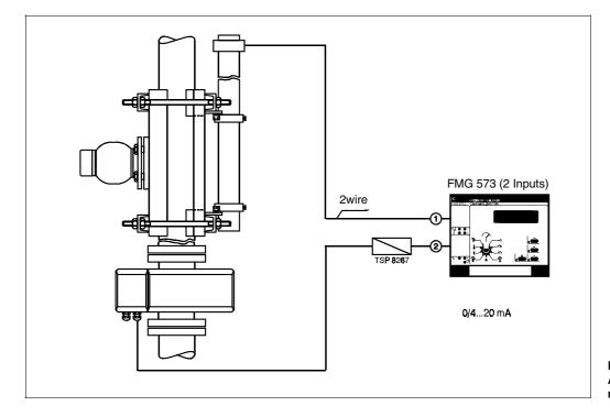
Fig. 4.1 Arrangement for mass flow measurement
