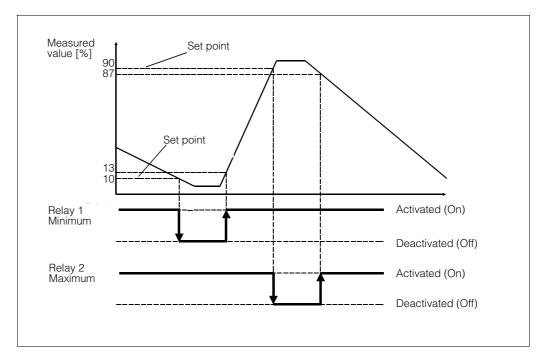
Fig. 3.10 Minimum and Maximum fail-safe mode
