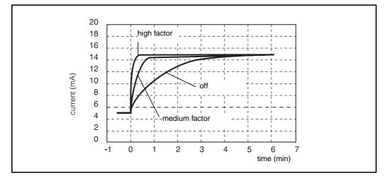
Fig. 7.1: Effect of damping factor
