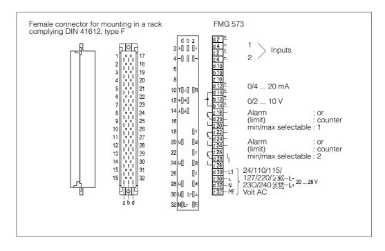
Fig. 3.2 Pin assignment and coding pins
