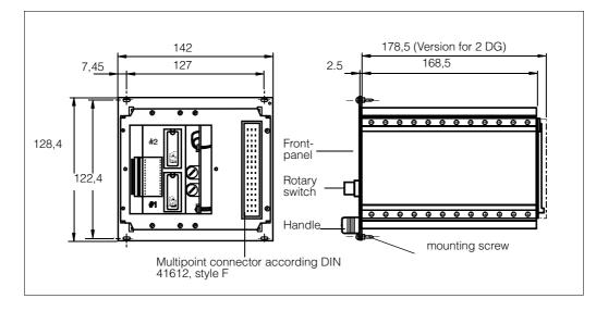
Fig. 1.9 Dimensions in mm transmitter FMG 573 Z/S
