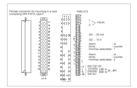
Fig. 4.2 Pin assignment and coding pins
