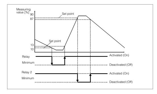
Fig. 5.12 Minimum and Maximum fail-safe mode
