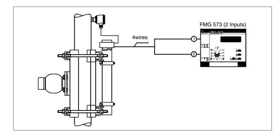
Fig. 5.1 Arrangement for temperature compensated density measurement with sensor TMT 2130 Z
