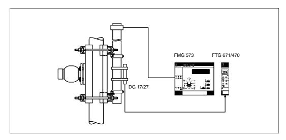
Fig. 1.10 Density measurement with radiation monitoring through FTG 671/470
