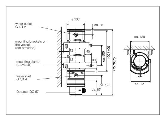
Fig. 1.8 Dimensions in mm detector DG 57 with water jacket
