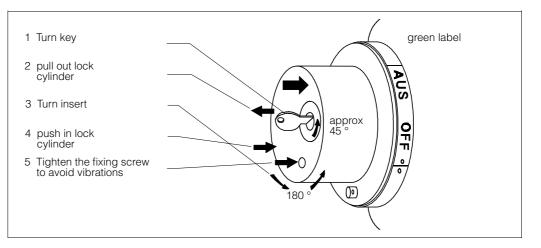
Fig. 2.6 Switch on
