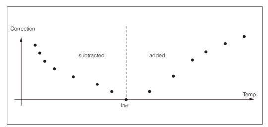
Fig. 1.1 Correction as a function of temperature
