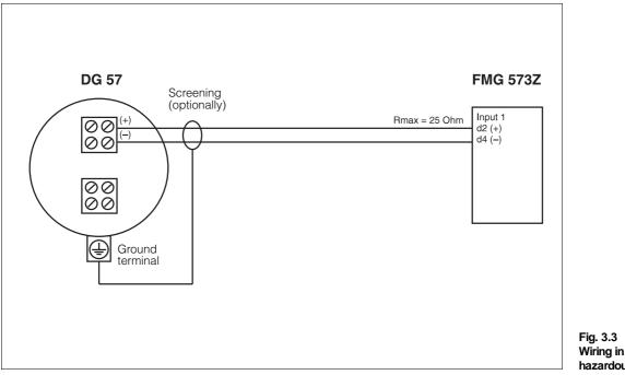
Fig. 3.3 Wiring in non-explosive hazardous areas
