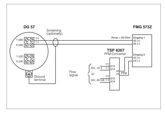
4.2.3 Wiring for non-explosion hazardous applications
