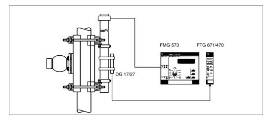
Fig. 3.1 Arrangement for density measurement
