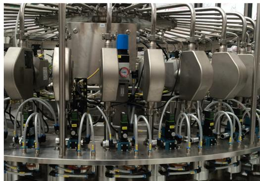
Rotary filling machine – equipped with Dosimass flowmeters
