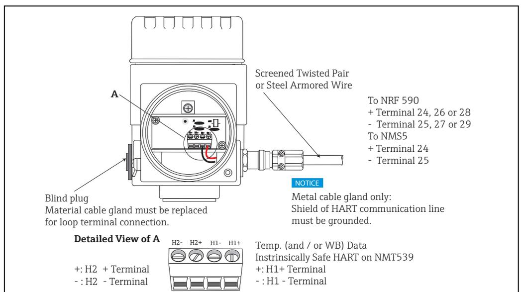
Figure 2: Description of Terminal Board
