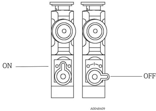
Figure 3. ON and OFF positions of the laser beam shutter
