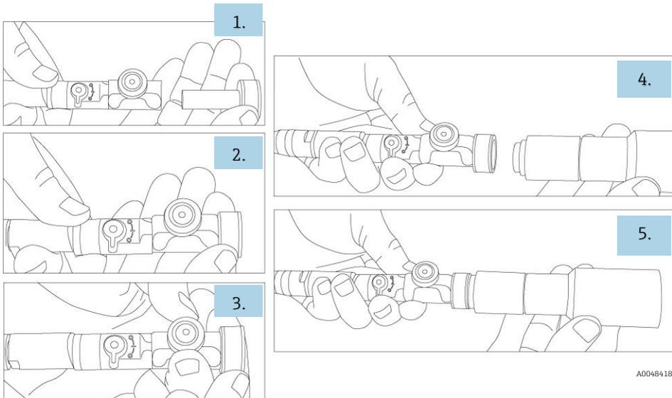
Figure 8. Installing an adapter and non-contact optic on an Rxn-10 probe
