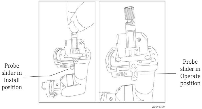
Figure 7. Verification accessory with probe slider in Install position (left) and Operate position (right)
