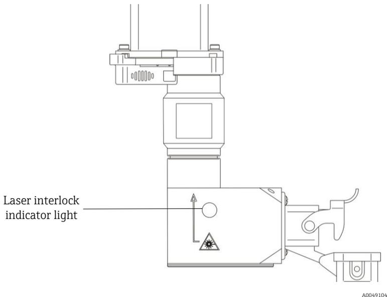
Figure 2. Location of laser interlock indicator light
