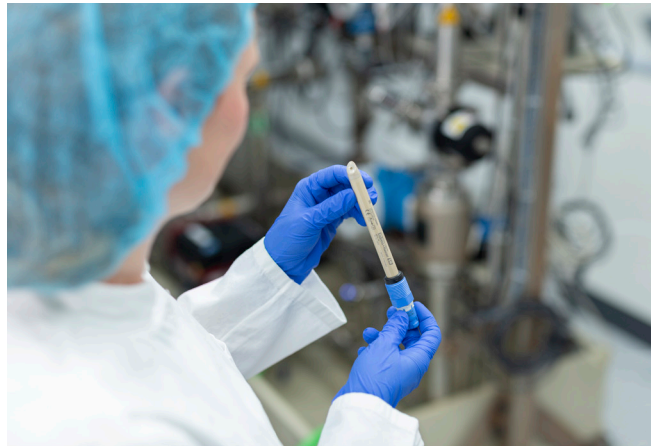
Memosens ISFET pH sensors are designed for hygienic applications
