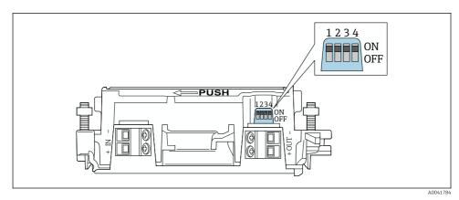
☑ 21 DIP switches for hardware-locking of functions
