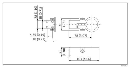
☑ 7 Dimensions of retaining bracket – wall mounting
