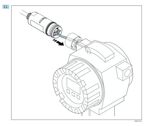
Ensure that the cores are of sufficient length to be connected in the field device. Shorten the cores in the field device to the required length.
