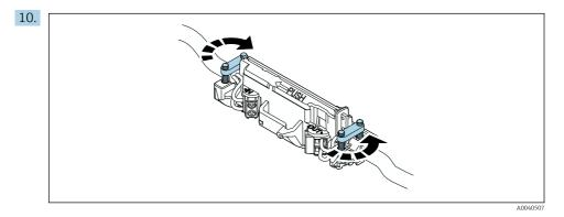
Tighten screws for strain relief. Torque: 0.4 Nm  $\pm$  0.04 Nm
