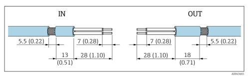
In Recommended dimensions for stripping in the case of cable glands for shielded cable for input terminal IN and output terminal OUT
