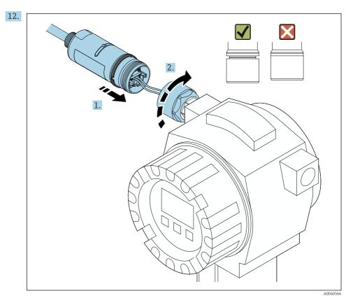
Do not tighten the top housing section yet, so that you are still able to rotate the bottom housing section.
