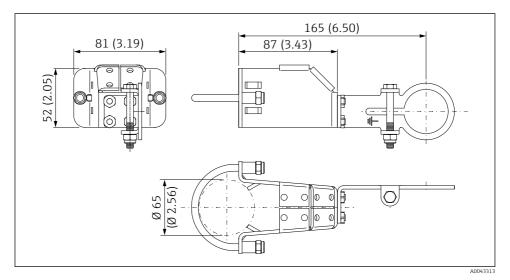
E 6 Dimensions of mounting bracket – pipe mounting
