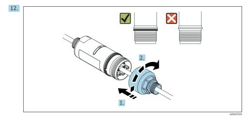
Tighten the top housing section so that the blue design ring can still be rotated afterwards. Torque: 5 Nm  $\pm$  0.05 Nm
