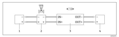
I3 Electrical connection for 4-wire HART field devices with active current output (optional grounding not shown) – PLC or transmitter at OUT terminals
