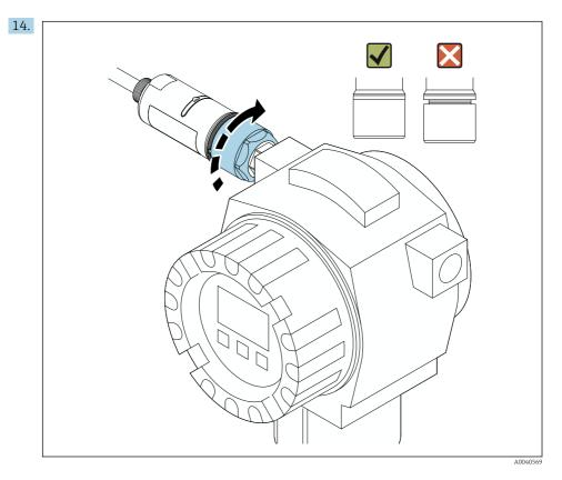
Tighten the top housing section so that the blue design ring can still be rotated afterwards. Torque: 5 Nm  $\pm$  0.05 Nm
