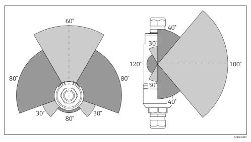
*■ 2 Different ranges depending on the position of the transmission window*
