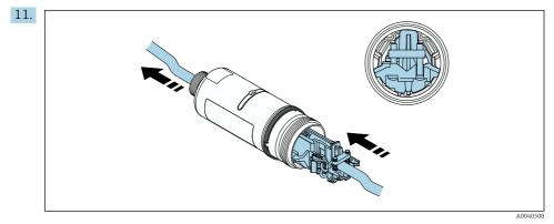
Slide the electronic insert into the guide inside the housing.
