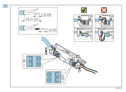
Ensure that the cores are of sufficient length to be connected in the field device. Do not shorten the cores to the required length until you are connecting them in the field device.
