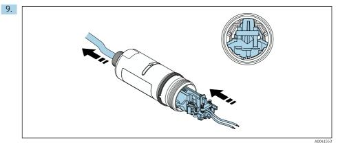
Slide the electronic insert into the guide inside the housing.
