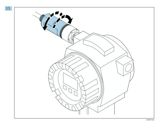
Align the bottom housing section with the transmission window according to the network architecture  $\rightarrow \implies 11$ .
