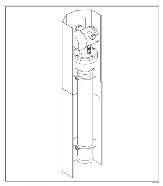
Example of a heat shield for Gammapilot FMG50
