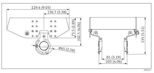
₹ 26 Weather protection cover for dual compartment housing, aluminum. Unit of measurement mm (in)
