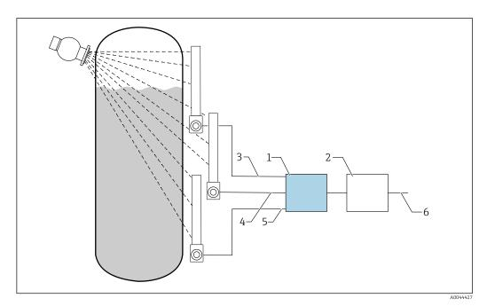
$Connection\ diagram: for\ three\ FMG50\ units\ (up\ to\ 20\ FMG50s)\ connected\ to\ one\ RSG45$ ₹ 25
