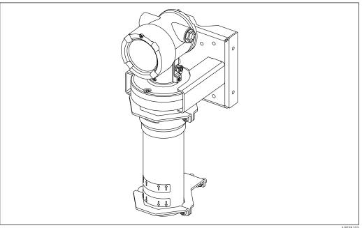
Installation overview, with mounting clamps and retaining bracket
