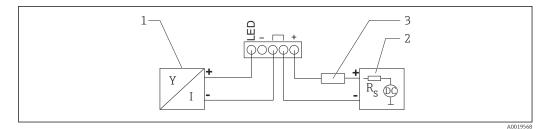
${ { { \Bbb B} } }$  6 Block diagram of HART device with RIA15 process indicator with light
