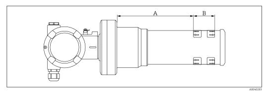
**№** 17 A defines the distance between the device flange and the start of the measuring range. Distance A depends on the material of the scintillator (PVT or Nal).
