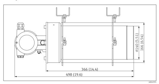
🖪 11 🛮 Version NaI (Tl) 2" with collimator on sensor side
