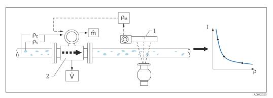
Mass flow measurement (m) using a density meter and a flowmeter. If the density of the solids  $(\rho_s)$  and the density of the carrier liquid  $(\rho_c)$  are also known, the solids flow rate can be calculated.
