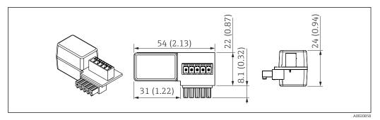
■ 24 Dimensions of HART communication resistor, engineering unit: mm (in)
