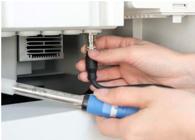
Easy connection with M12 connector
