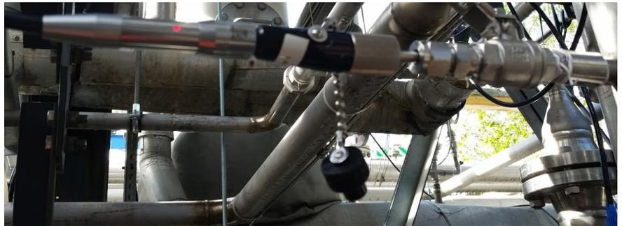
In-line chemical analysis of amine process stream by a Raman immersion probe at the CO<sub>2</sub> capture plant facility in Sheffield, UK
