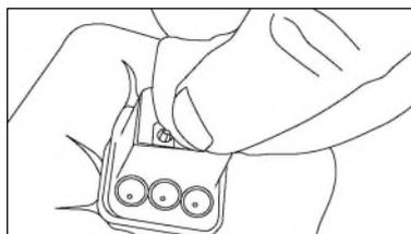
Figure 3. Cleaning electro-optical fiber connection
