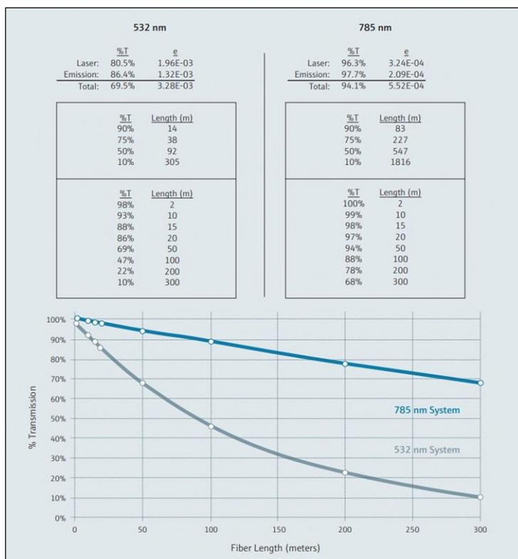
Figure 5. Measured fiber transmission (%T) vs. fiber length
