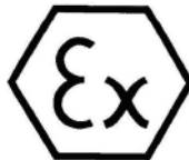
Figure 1. ATEX label for use in hazardous areas
