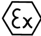
Figure 4. ATEX label for use in hazardous areas
