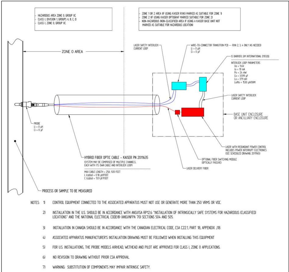
Figure 11. Hazardous Area Installation Drawing (4002396 version X4)
