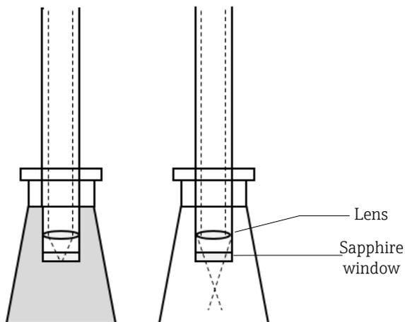
Figure 7. Use of Rxn-40 probe with short (left) vs. long (right) data collection zone
