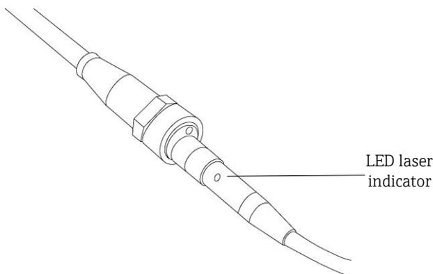
Figure 2. LED laser indicator on integrated stainless steel fiber connection shell
