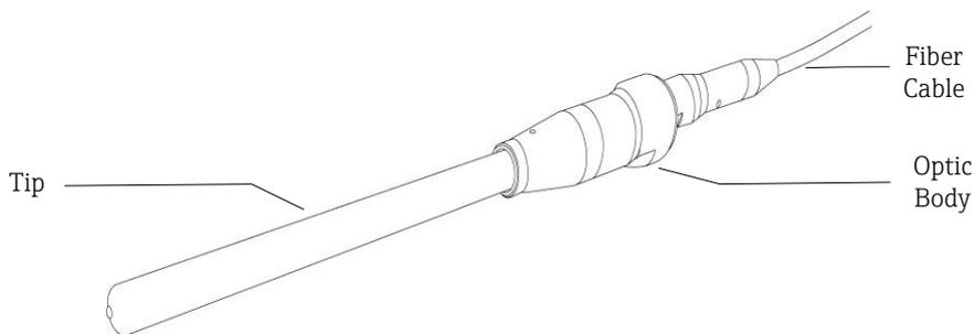
*Figure 4. Non-flanged configuration of the Rxn-40 probe*
