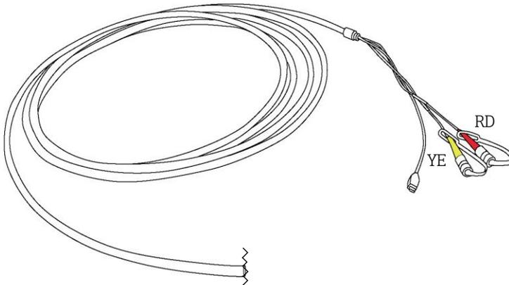
Figure 9. FC cable assembly showing connector for analyzer
