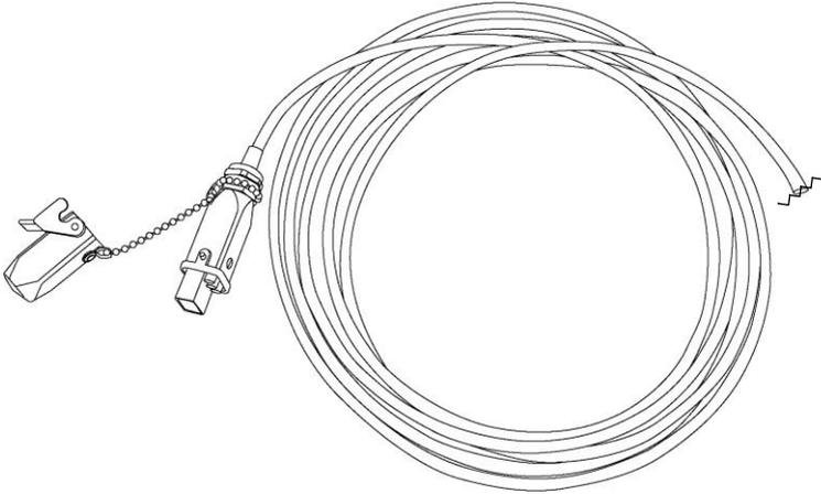
*Figure 10. EO fiber cable showing connector for analyzer*
