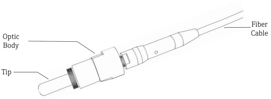
Figure 6. Mini configuration of the Rxn-40 probe
