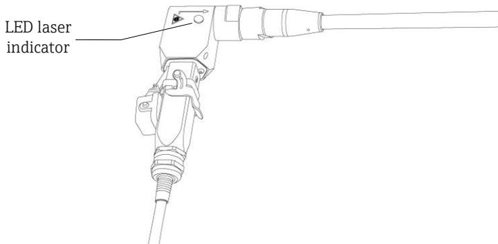
*Figure 3. LED laser indicator on right-angle fiber connector (EO style) assembly*
