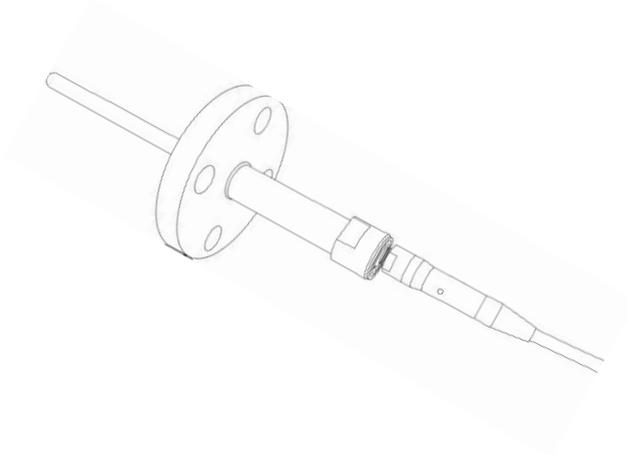
Figure 5. Flanged configuration of the Rxn-40 probe
