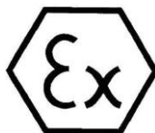
Figure 2. ATEX label for use in hazardous areas
