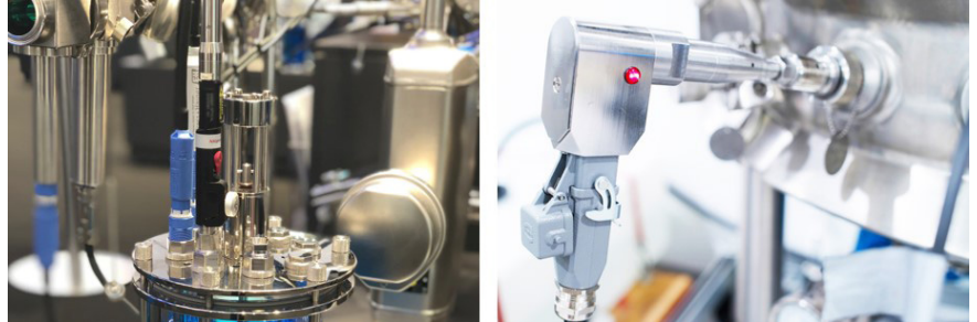
Figure 1: Real-time, in situ probes, optimized for bioprocess conditions, enable measurements in laboratory (left) and manufacturing (right) with easy transfer of the analytical model.
