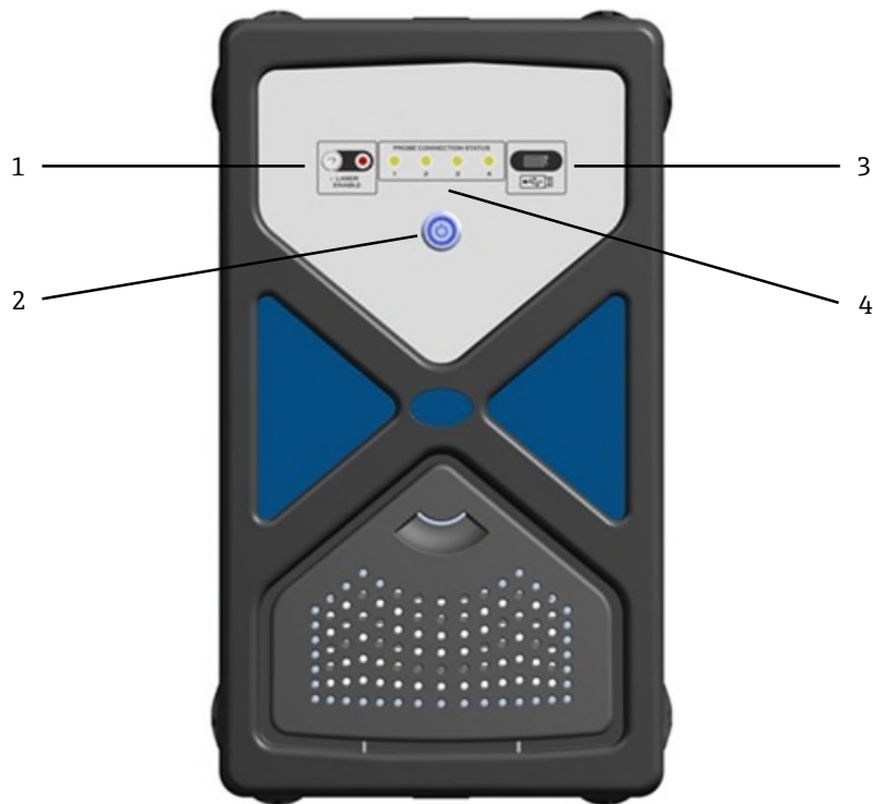
Figure 1. Front panel of a Raman Rxn2 four channel analyzer
