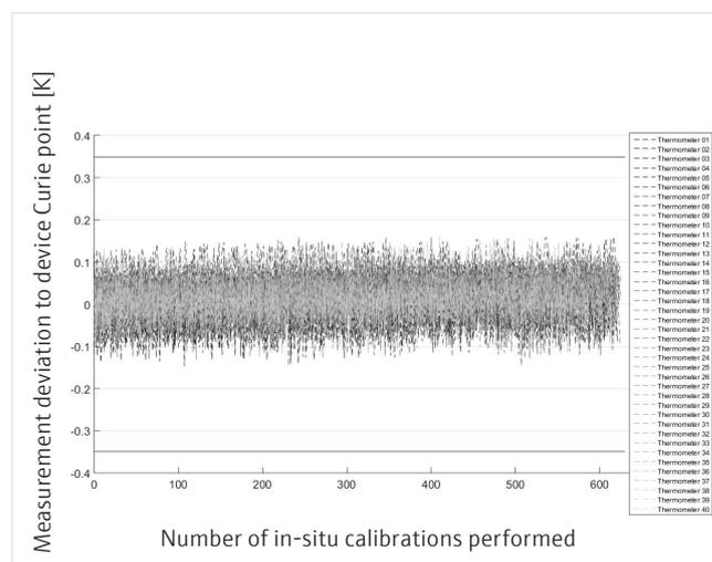
Fig. 4: Long-term analysis of detected measurement deviation at Curie point with 40 Endress+Hauser iTHERM TM371 (Source: TÜV Thüringen)
