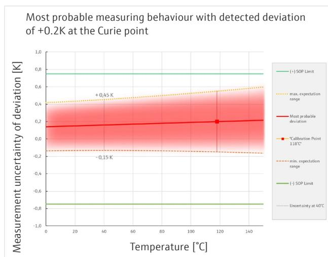
Fig. 3: Measurement uncertainty analysis of single-point calibration
