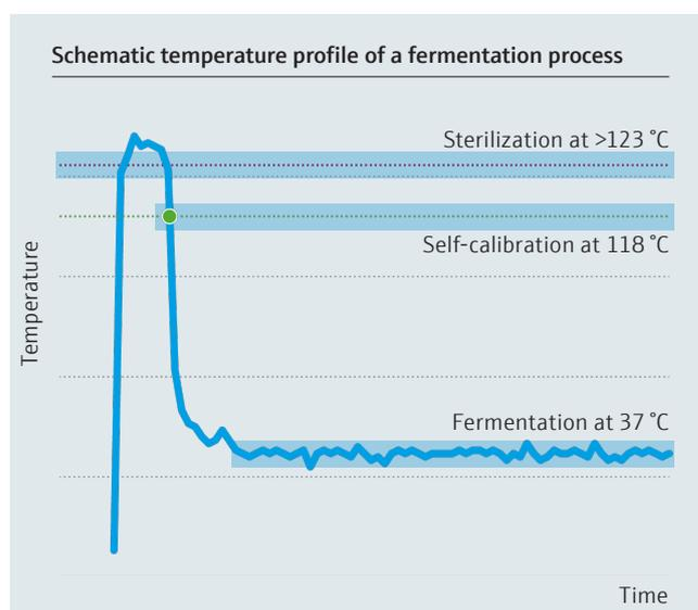
Fig. 2: Typical temperature graph based on the example of a fermentation process
