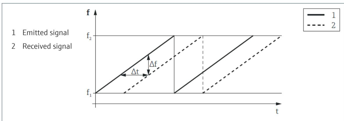
Figure 3: FMCW principle: Results of the frequency modulation
