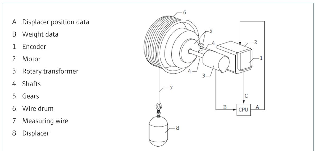
Figure 1: Proservo NMS8x Measuring Technology
