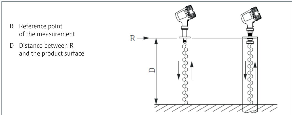
Figure 2: FMCW principle: Emission and reflection of the continuous wave
