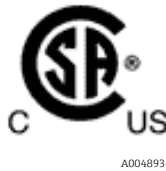
Figure 4. CSA label for use in hazardous areas in the US and Canada
