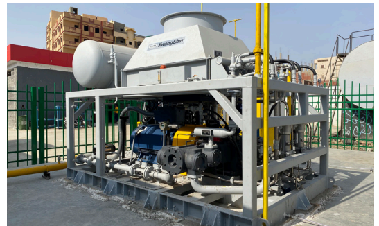
Compressor model: GEO-BII 200HP 4stage, Electric motor driven CNG Compressor delivered in Egypt
