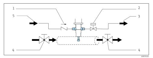
■ 14 Example of a sealing system via a bypass.
