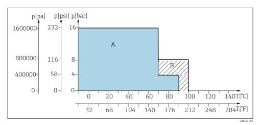
■ 57 Pressure/temperature ratings for basic version for materials PVDF and PVDF conductive (CPA871-\*\*\*\*\*E/F\*\*\*\*)
