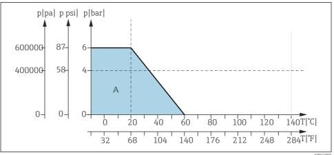
Pressure/temperature ratings for basic version for the material PP (CPA871\-\*\*\*\* $H^{***}$ ) **■** 51
