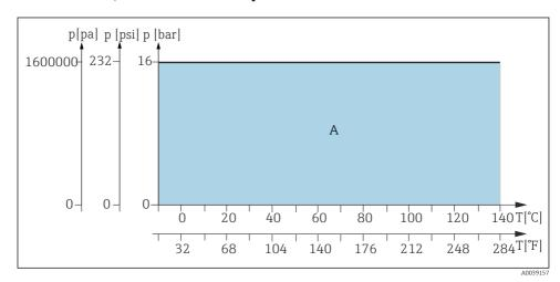
■ 56 Pressure/temperature ratings for basic and immersion chamber version for materials 1.4404, Alloy C22 and PEEK (CPA871-\*\*\*\*E/F\*\*\*\*)
