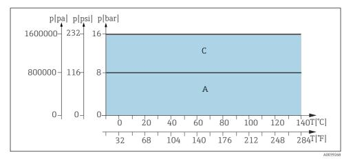
54 Pressure/temperature ratings for basic and immersion chamber version for materials 1.4404, Alloy C22 and PEEK (CPA871-\*\*\*\*\*G/H\*\*\*\*)
