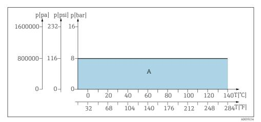
■ 52 Pressure temperature ratings for basic and immersion chamber version for materials 1.4404, Alloy C22 and PEEK
