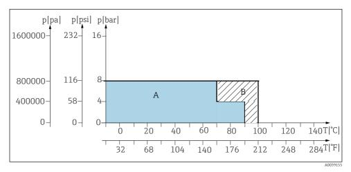
$\blacksquare$  53 Pressure temperature ratings for basic version for materials PVDF and conductive PVDF
