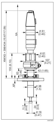
■ 8 Immersion chamber version with pneumatic drive, dimensions in mm (in)
