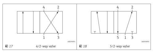
Connection 1 is attached to the compressed air supply.
