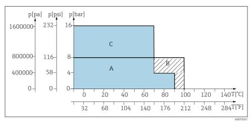
55 Pressure/temperature ratings for basic version for materials PVDF and PVDF conductive (CPA871-\*\*\*\*\*G/H\*\*\*\*)
