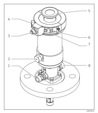
■ 1 Assembly with pneumatic drive (without protective cover)
