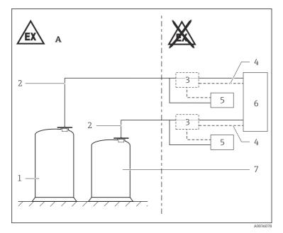
Electric connection of two sensors Prosonic FDU9x to the analysing unit Prosonic S
