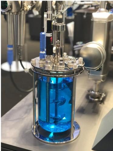
The Rxn-10 and bIO-Optic used in advanced bioprocess control
