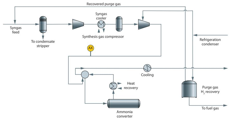
Figure 1: Typical ammonia converter feed measurement point\*
