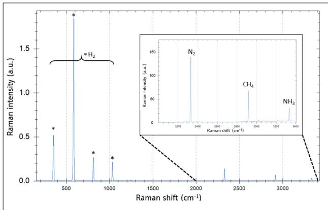
Figure 2: Raman spectrum of a typical ammonia converter feed stream
