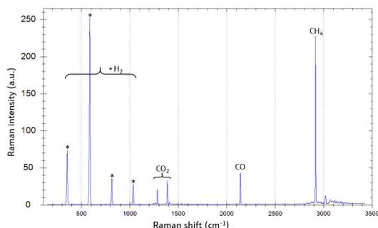
Figure 2: Typical Raman spectrum for syngas
