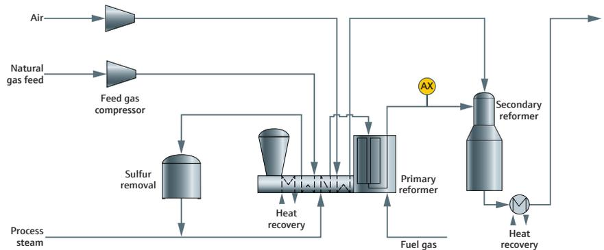
Figure 1: Primary steam reformer section of HyCO plant process units\*\*
