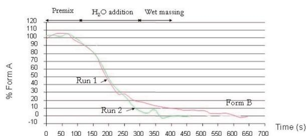
Figure 2: Predicted form conversion, form A to B. In Run 1, the chopper was turned on after water addition. In Run 2, the chopper was on during and after water addition. (Reprinted with permission from Ref. 1. © 2006 Russell Publishing.)
