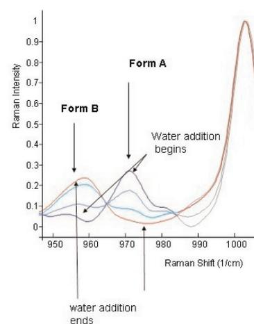
Figure 1: Raman spectral change during HSWG polymorph transformation. (Reprinted with permission from Ref. 1. © 2006 Russell Publishing.)
