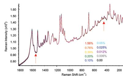
Figure 1: Raman spectra of furosemide tablets with various degradant content
