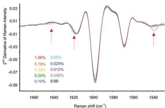
Figure 2: Second-derivative treatment of the tablet spectra
